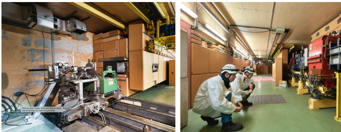
Figure 1 The antiproton decelerator target region and its associated shielding blocks.
