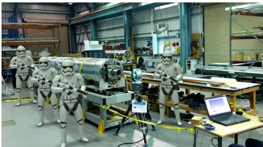
Figure 1 Measurement test bench for a very precious high-luminosity LHC magnet.
